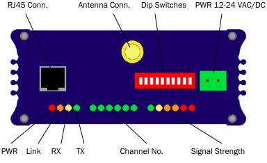
Operating Voltage: 12-24 VAC/DC (not polarity sensitive) Power Consumption at Max Power: 200mA @ 12VAC/DC
